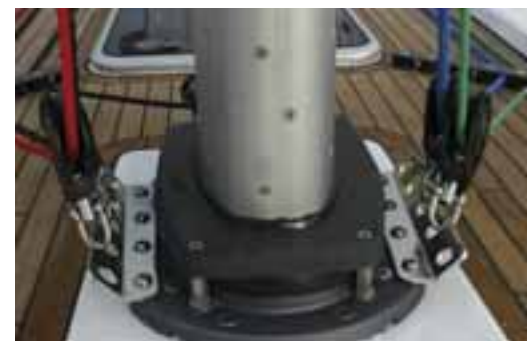
Deck collar including wedging and deck waterproofing, as well as the halyard blocks for keel stepped masts.
